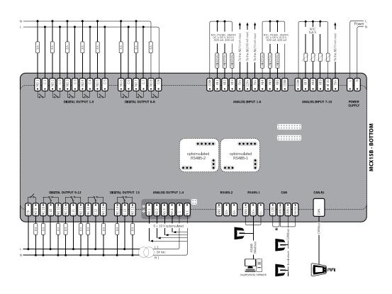
\*NOTE: connection has to be made on the first and last local network units, make the connection as close as possible to the connector \*\*NOTE: optoinsulated analog outputs voltages are referenced to contact N1
